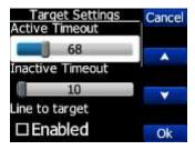
With **Edit** you can activate slider control, then **up/down** buttons you can select the preferred value and confirm it with the **Ok** push button.
