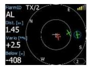
Middle buttons help with target selection by cycling through available targets. Lower button has EDIT function, where we can edit/view the currently selected target.
