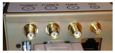
FLARM A and B Ports are reverse polarity female SMA connectors, with a (male) pin as centre conductor. ADS-B is a standard female SMA connector with a female centre receptacle.
